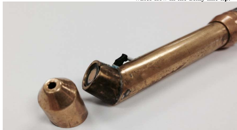
Figure 3.7 The fabricated UDS probe with the tip cup (delay line for coupling fluid).
